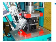
Crimp and Bend module option is ideal for single parts with bends up to 45 degrees. Combine crimping and bending into one operation with this time saving option.
