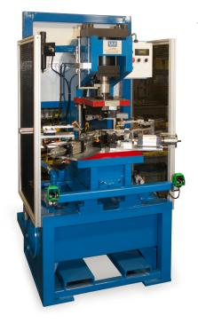
Machine guarding options include: Wire mesh, Lexan, horizontal and vertical light curtains.
