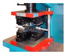
Single and double hose insertion and double crimp within single die set combines multiple task in one operation.
