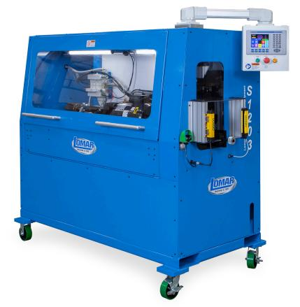
The Operator Interface Screen has the ability to store multiple part numbers enabling the operator to make simple part to part changes including diameter changes from 5/16" to 3/4" diameter tubing when utilizing the same roll form configuration.
