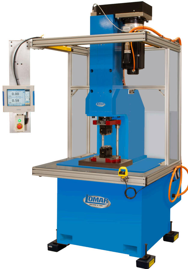
Shown with optional 3-section light curtains and side mounted servo unit.
