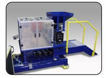
Bowl feeder load systems accommodate a wide range of parts for assembly processes.
