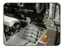
Tube Hoppers accommodate a wide range of tube diameters and lengths.
