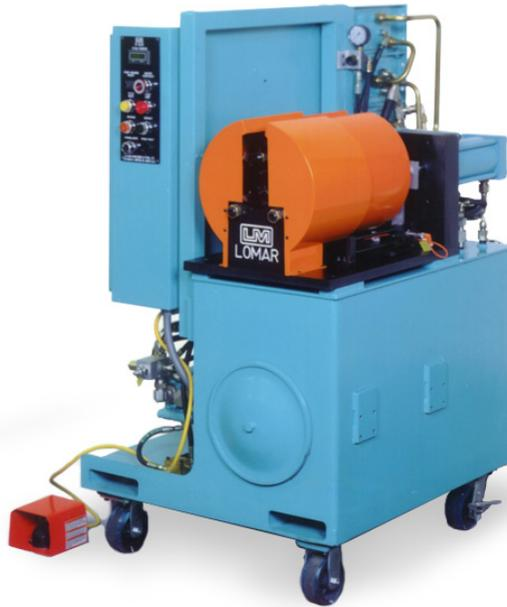
The powerful Lomar S1133 high production crimp machine adapts especially well to crimping operations that require attaching bent or long tubes to hose.
